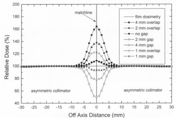
**Figure 5.** Relative dose profiles at the junction. Solid line shows the profile of film which is seen in Figure 1.
