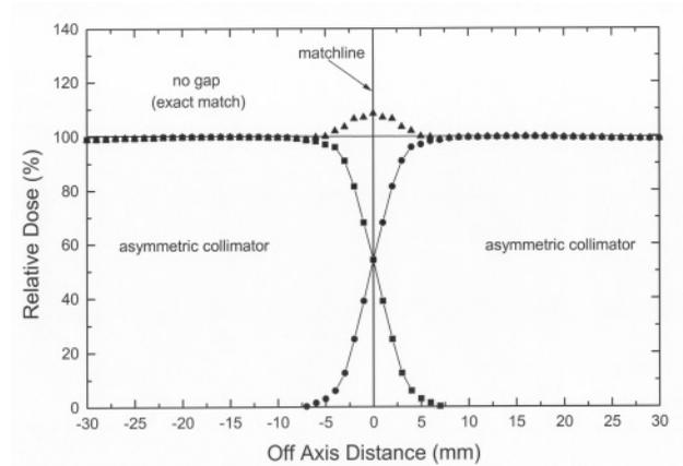
**Figure 4.** Composite dose profile of two asymmetric fields obtained by mathematical summation for exact matching (no gap).
